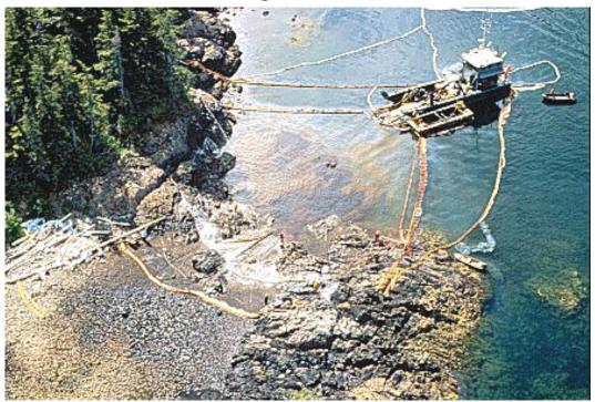
Booms and skimmers worked poorly. Booms are floating "sausages" with skirts that hang a few feet below the surface. They corral the "pancake" of floating oil. Skimmers then collect the oil by sucking or scooping it up. But there was too much oil and not enough equipment. Some of the skimmers jammed or broke. (See SW May 19, 1989, page 3, Teachers' Edition, for more detail on the various cleanup methods.)
