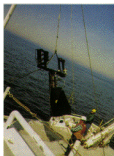
The Video Plankton Recorder sends back images, that for the first time, let scientists observe microscopic life forms, undisturbed, in their natural environment.
