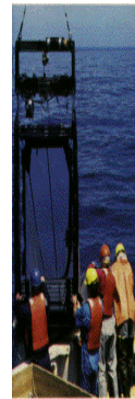
The MOCNESS net system brings back samples from many different water levels
