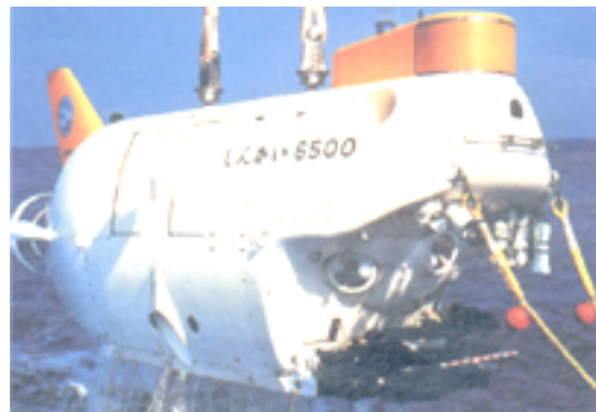
JAMSTEC's Shinkai 6500 is two meters longer than ALVIN, and carries two pilots and one scientist, rather than one pilot and two scientists.
